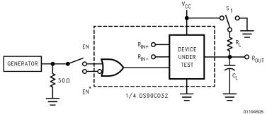
$\mathbf{C}_{\mathsf{L}}$  includes load and test jig capacitance.
