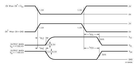
FIGURE 4. Receiver TRI-STATE Delay Waveforms
