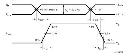
FIGURE 2. Receiver Propagation Delay and Transition Time Waveforms
