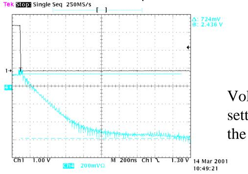
Voltage controlling delay settles 2µs after reset of the circuit
